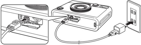
Connect the camera using the supplied Micro USB cable to a USB AC adapter (supplied with your smartphone) then connect the USB AC adapter to an indoor power outlet.
