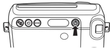
Press the POWER button to turn the camera on.
