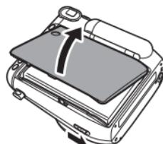
Press down the back cover lock to open the back cover.
