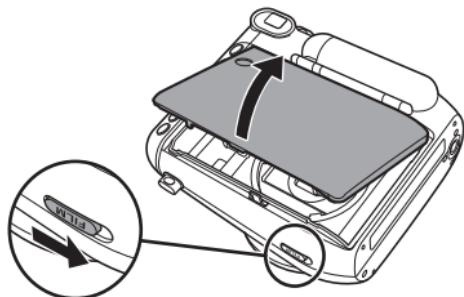
Press down the back cover lock to open the back cover.
