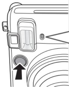
If you press the shutter button, the self timer lamp is lit about 7 seconds. After that, the lamp flashes about 3 seconds and the shutter is released.
