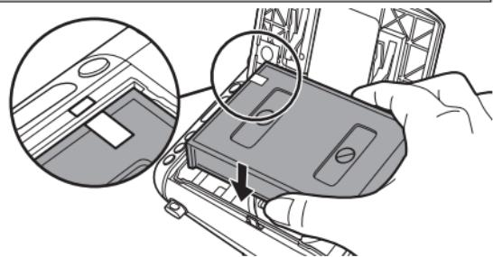
Hold both sides of the film pack, align the yellow marks on the camera and the film pack, then insert it straight.
